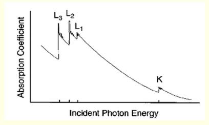
■ XAS: given by the ℓ±1 partial DOS of the conduction bands of the specific atom (with core state ℓ) times the TME<sup>2</sup>
